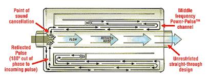
creates sound waves 180 degrees out of phase with the exhaust noise. This design cancels unwanted frequency's and let's through the desirable exhaust notes. In addition, the gas path through the muffler is straight through (like a glass pack) with no restrictive baffles.
